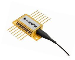
The 808nm series laser diodes are fabricated in a hermetically sealed 14-pin butterfly package. The laser diodes contain a monitor photodiode, thermoelectric cooler (TEC), and a thermistor to secure high-quality laser performance. Our laser products are Telcordia GR-468 qualified and in compliance with RoHS Directives.
